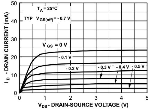
Figure 6. Common Drain-Source
