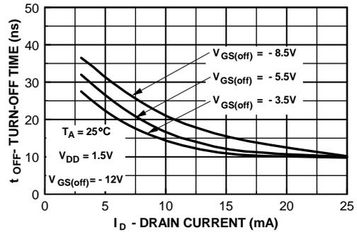
Figure 10. Switching Turn-On Time vs. Drain Current
