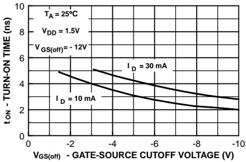
Figure 9. Switching Turn-On Time vs. Gate-Source Cut-Off Voltage
