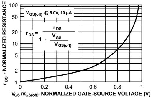
Figure 7. Normalized Drain Resistance vs. Bias Voltage
